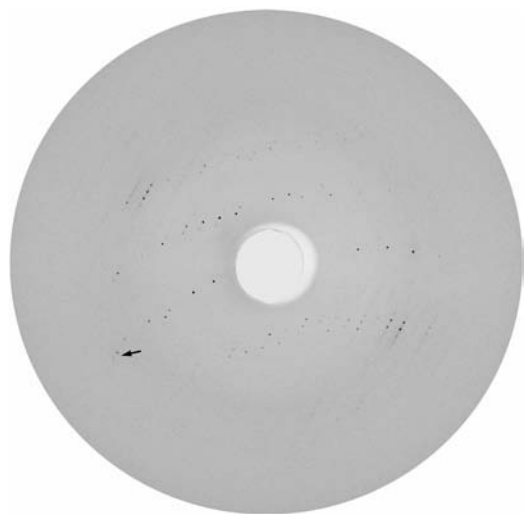
Figure 3 X-ray diffraction pattern of a single crystal of CcpA in complex with 17 TA. The image was recorded using the X-ray beam at beamline X11 (EMBL Outstation, Hamburg) on a MAR Research imaging plate with an oscillation angle of 2°. The arrow corresponds to 8.5 Å resolution.
